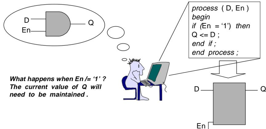
If you intend to simply gate a input signal with a control or enable, you must specify the appropriate “else” statement assigning ‘0’ to the output.
