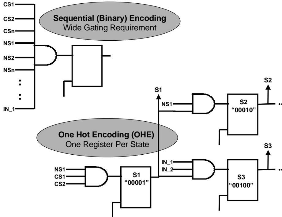
**Figure 14. Sequential Encoding Vs. One Hot**
