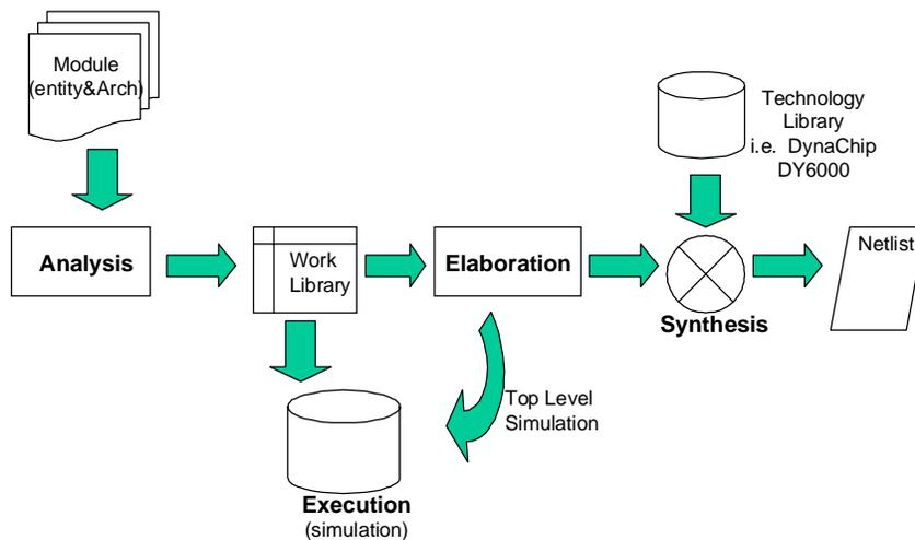
**Figure 5. The Synthesis Compilation Process**
