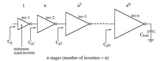
Each driver (inverter) larger than preceding driver by stage ratio "a".
