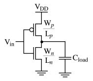
For  $t_{fall}$ , would expect NAND gate to be twice as slow (as the base inverter) because channel lengths add.
