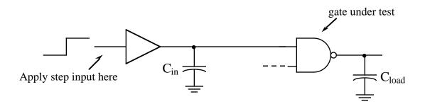
Vary  $C_{in}$  to control input slope. Only problem is that precise control of input slope is difficult, must be able to accurately predict slope of output gate based upon value of " $C_{in}$ ".
