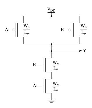
In delay terms (for this NAND), for  $t_{rise}$ , would expect to have the <u>same</u> worst <u>case</u>  $t_{rise}$  as the base inverter because either A or B *p*MOS will pulling.
