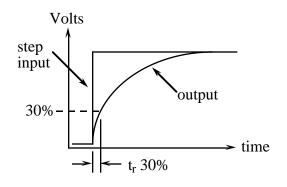
Delay can be modeled in terms of an <u>RC</u> delay:
