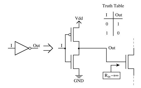
Note: Ideally there is <u>no</u> static power dissipation. When "I" is fully is *high* or fully *low*, <u>no</u> current path between Vdd and GND exists (the output is usually tied to the gate of another MOS transistor which has a very high input impedance).
