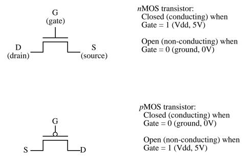
For *n*MOS switch, source is typically tied to ground and is used to *pull-down* signals:
