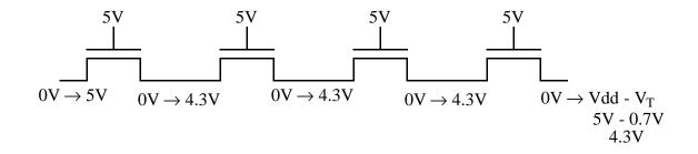
Only one threshold voltage drop across series of nMOS transistors
